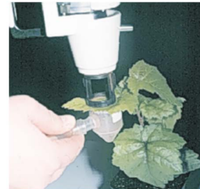
Figure 1. Bombarding birch leaves with the Helios™ Gene Gun.
